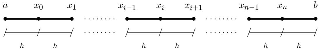
$$x_i = a + (i + 1)h, \quad f_i = f(x_i), \quad \text{para } i = 0, \dots, n; \quad h = \frac{b - a}{n + 2}.$$
