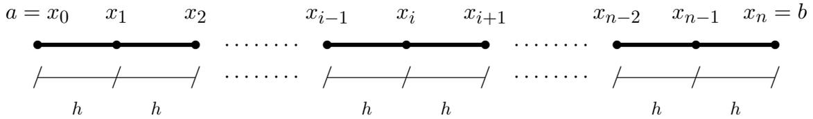
$$x_i = a + i h, \quad f_i = f(x_i), \quad \text{para } i = 0, \dots, n; \quad h = \frac{b - a}{n}.$$
