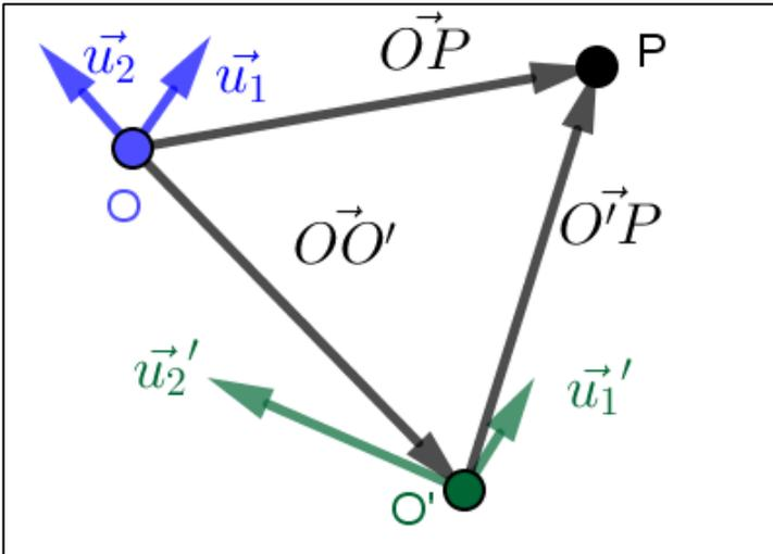
$$\begin{pmatrix} x_1 \\ x_2 \\ \vdots \\ x_n \end{pmatrix}_R = \begin{pmatrix} a_1 \\ a_2 \\ \vdots \\ a_n \end{pmatrix}_R + M_{BB'} \begin{pmatrix} x'_1 \\ x'_2 \\ \vdots \\ x'_n \end{pmatrix}_{R'}$$
