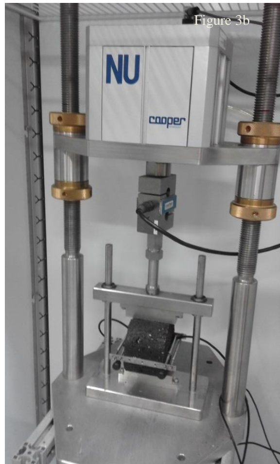
Figure 3: a) Marshall cylindrical specimen and b) Cooper NU14 servo-pneumatic machine.
