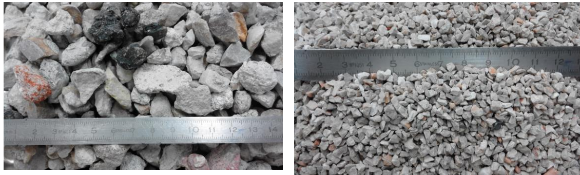
Figure 1. Aggregates used in this investigation: a) fraction 8/16 mm of RCA, with an 89.3% mix of concrete, stone or similar material and b) fraction 2/4 mm of limestone used as natural aggregate.
