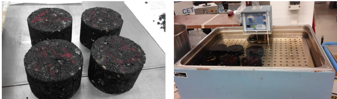
Figure 5. Water resistance test: a) “dry” subset at room temperature and b) “wet” subset in a water bath at 40°C.
