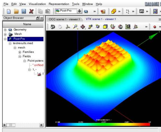
Figure 4. TOTBEM: 3D view of computed potentials on the ground surface.
