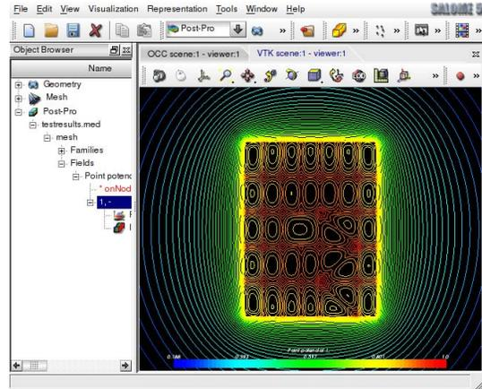
Figure 5. TOTBEM: Visualization of isopotential lines on the ground surface.
