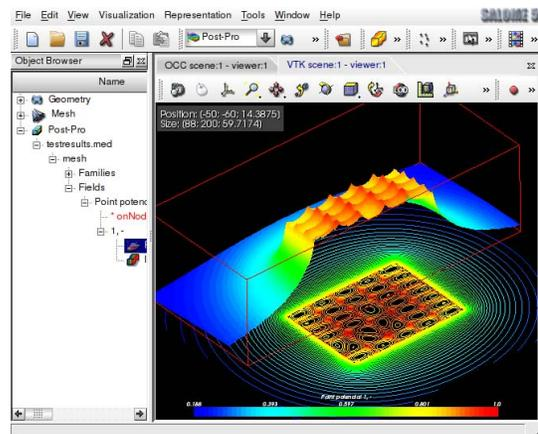
Figure 6. TOTBEM: 3D view of potential and isopotential lines.
