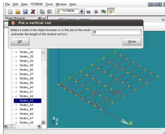
Figure 2. TOTBEM: Example of the input data for vertical rods.
