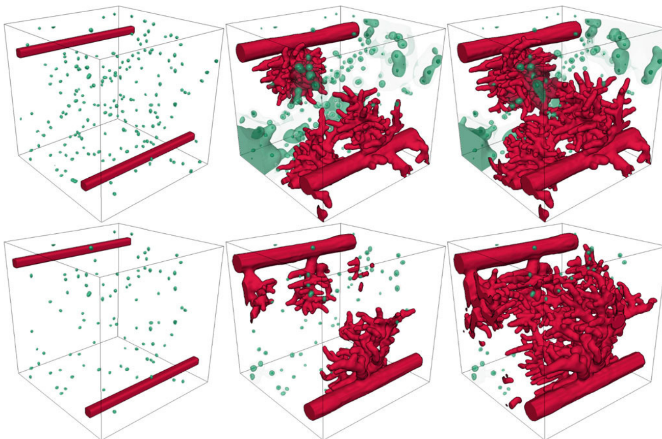
Fig. 7 Formation of two vascular networks with disguising characteristics. The capillaries in the first simulation (the three snapshots in the upper row) promoted by 200 hypoxic cells are thinner than those in the
